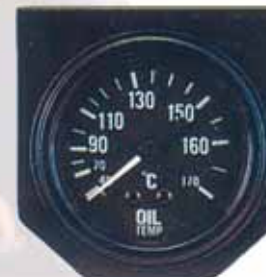
Model G-4005 Oil Temp. Gauge 40-170°C or 100-340°F 72" Capillary tubing & 1-1/2" adaptor
